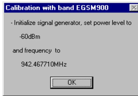
Connect an external signal generator to the RF connector of the phone and set the generator as told in the window, taking care for external cable losses.
