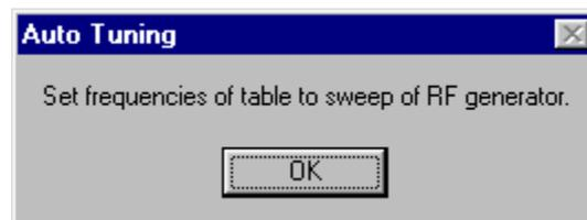
Connect an external signal generator to the RF connector of the phone and let the signal generator step sweep through the programmed frequency list.
