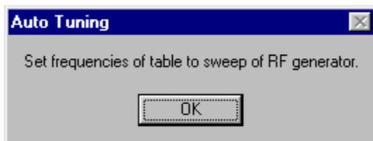
Connect an external signal generator to the RF connector of the phone and let the signal generator step sweep through the programmed frequency list.
